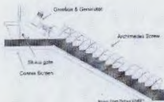
Gambar 1. Skema turbin ulir (Lakeside Equipment).
